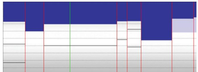
**Detailed Construction** reporting is designed to provide the Pavement Engineer with maximum level of information from a traffic speed survey. Unlike summary construction reporting, detailed construction provides you with statistical layer thicknesses, typically every half a meter.
